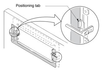
1-4. Clamp the wall or ceiling panel using the two board clamps, and secure with the clamp screws.
