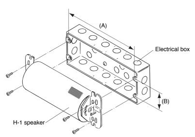
**Memo** Electrical box mounting screws are attached to the H-1 speaker.
