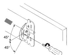
3-3. Align the two securing clips on the Trim Piece with the speaker's two stud screws, then push the Trim Piece onto the speaker until the Trim Piece is snug to the wall or ceiling surface.
