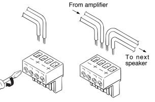
2-4. Attach two impedance selector sockets to the connector to select the desired impedance. Preset to 830  $\Omega$  (12 W for 100 V line and 6 W for 70 V line).
